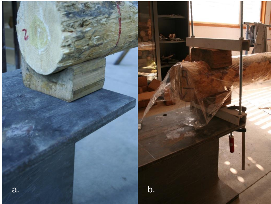
Figure 3: Support Types: a) Method A b) Method B
