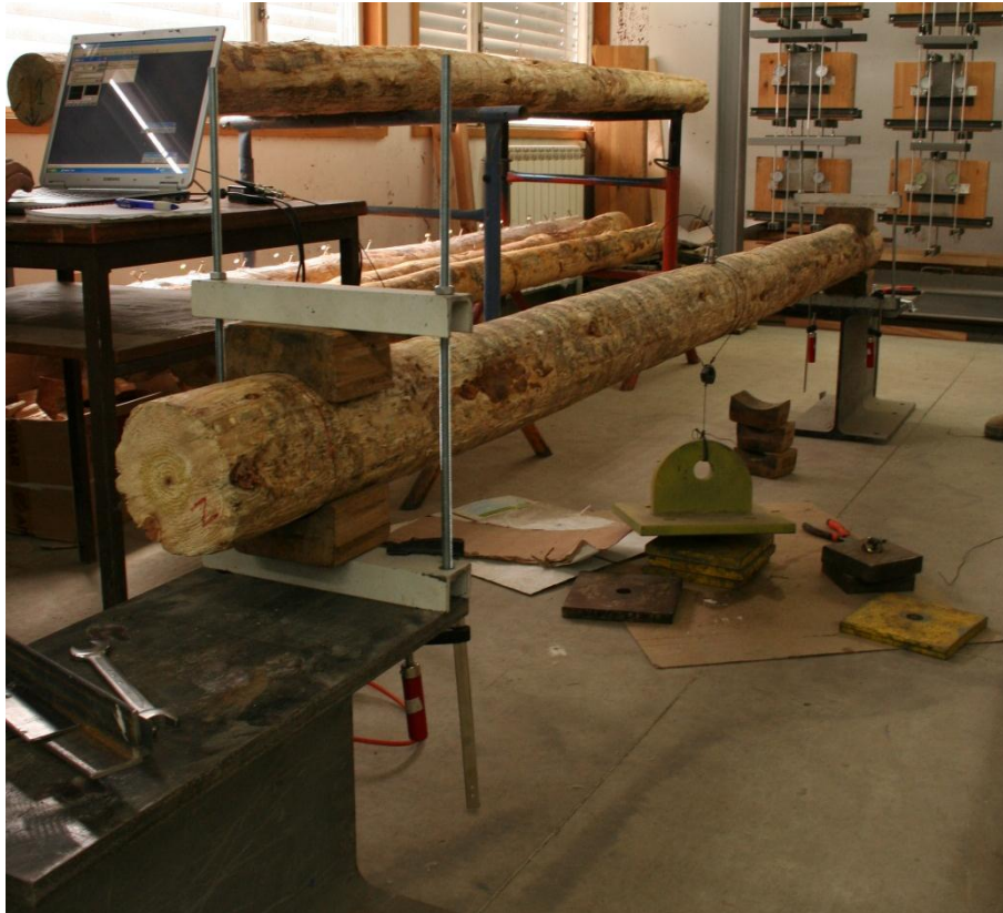
Figure 2: Timber Beam, Vibration Test Arrangement
