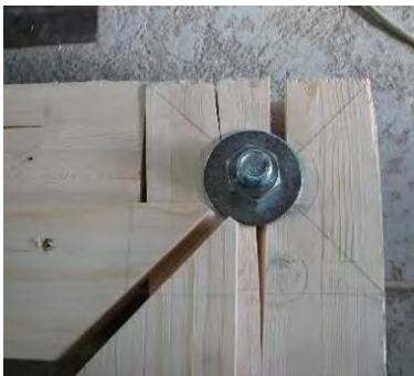
Fig. 6 Failure when one screw was used Fig. 7 Joints with screw and punched nailed plate
