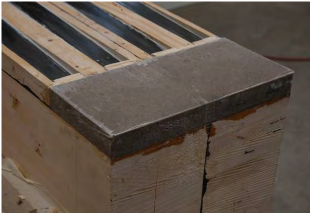
Fig. 4 End-anchorage of the CFRP-lamella / Bearing
