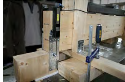
(iii) Reinforcement with screwed steel plates
