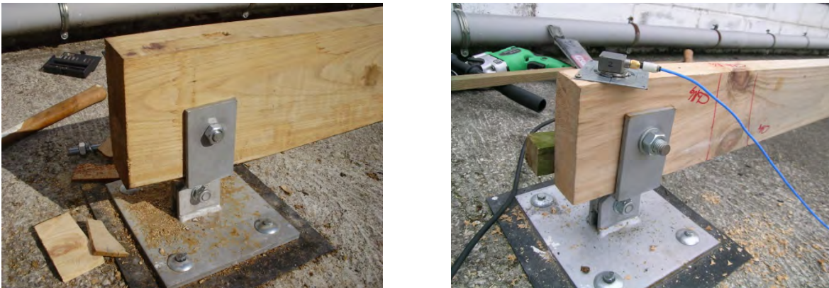
Figure 3. Test for pinned-pinned supported beams.
