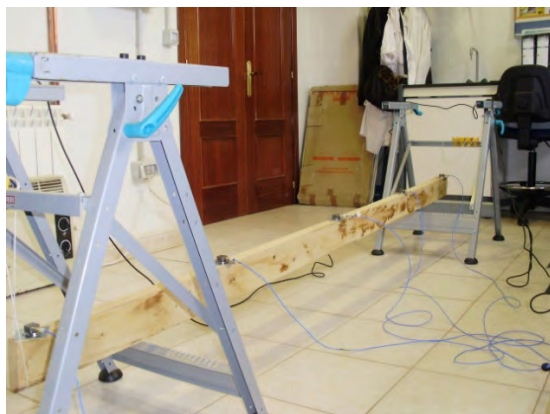
Figure 1. Test for hanging beams (free-free condition).
