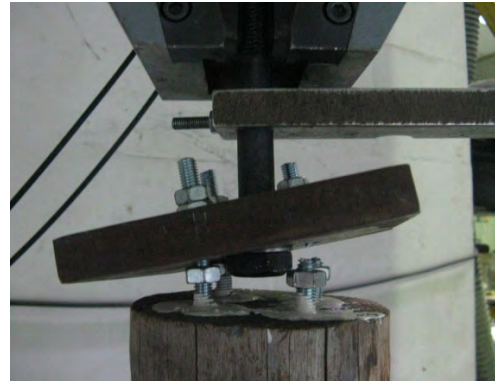
Fig. 6 Failure of a connection
