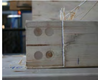
(ii) Reinforcement with glued-in birch rods
