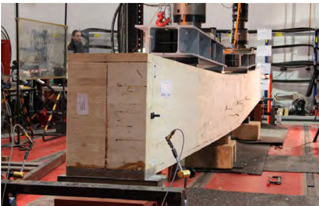
Fig. 1 Specimen in test after tensile-failure of the wood
