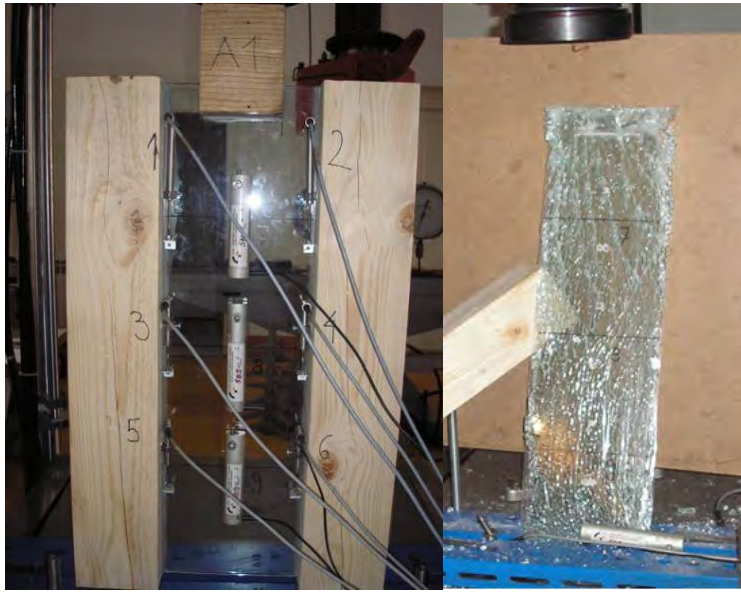
Fig. 1 Shear test on composite system timber-glass obtained by gluing and type of failure
