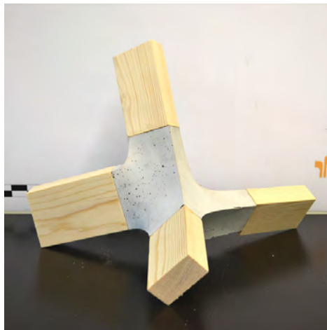
Fig. 9 Concrete Joint connected to timber
