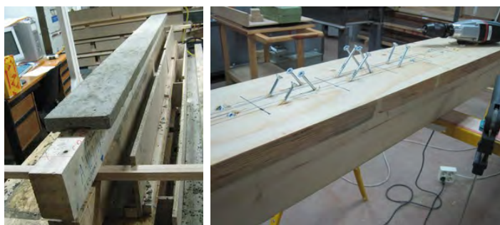
Fig. 1 a) glulam-concrete and b) glulam-LVL composite joist
