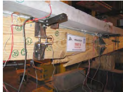
Fig. 14 Collapse of the beam
