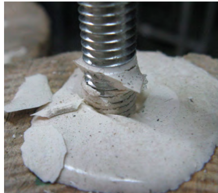
Fig. 4 Failure in the glue
