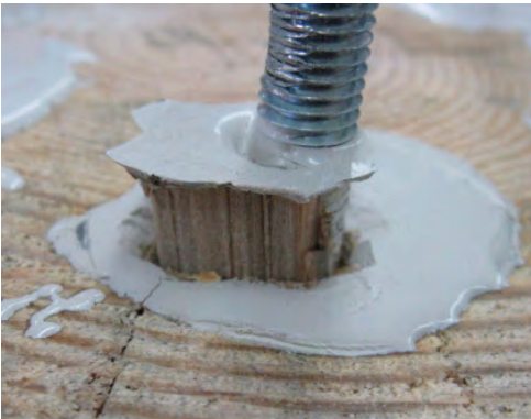
Fig. 3 Failure in the wood
