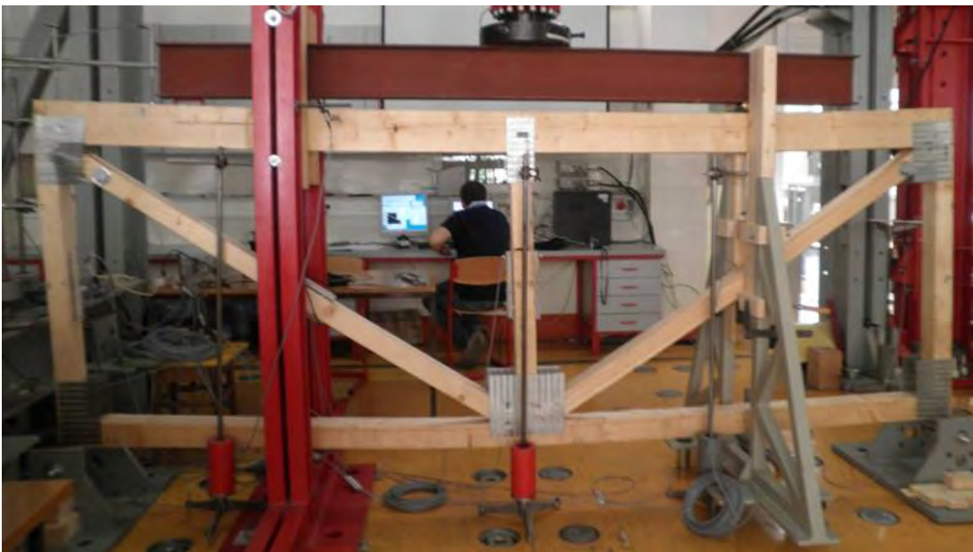
Fig. 3 Truss system with punched metal plates.
