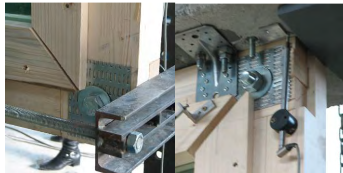
Fig. 6 Failure when one screw was used Fig. 7 Joints with screw and punched nailed plate
