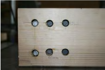
(i) Reinforcement with glued-in threaded steel rods
