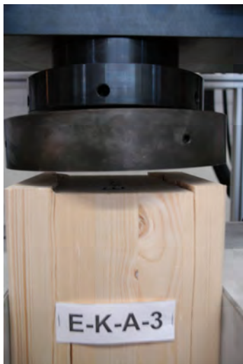
Fig. 5 Failure due to shearing of timber in front of the joint
