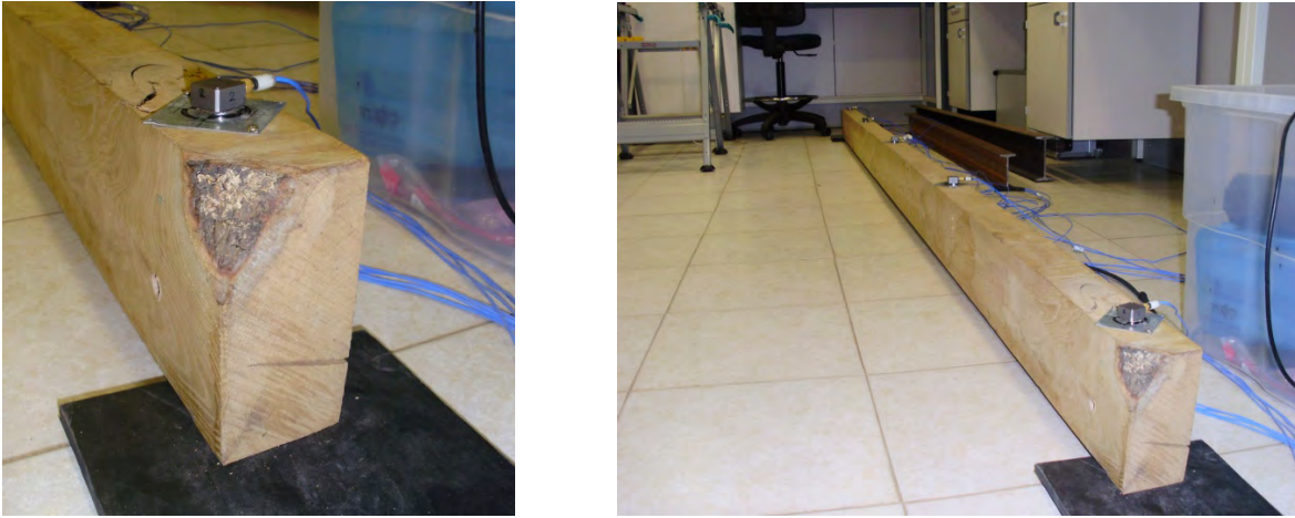
Figure 2. Test for simply supported beams on neoprene.
