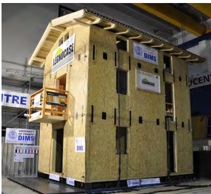
Fig. 7 Full-Scale timber building shake table test
