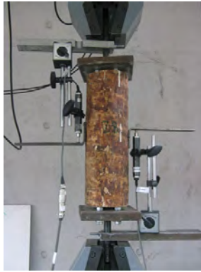
Fig. 5 Test arrangement of the connections
