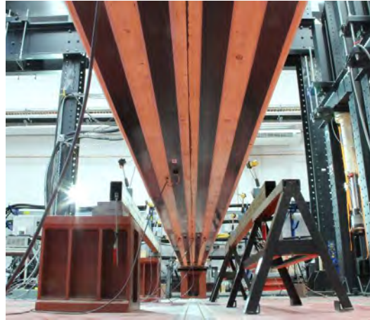
Fig. 3 Tension Zone of the HTB reinforced with CFRP-lamellae
