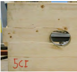
Fig. 4 Typical shear plug failure
