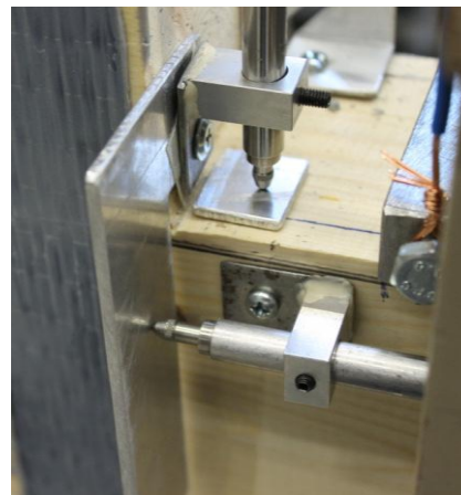
Figure 5: Application of LVDT measurement sensors
