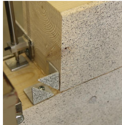
Figure 6: Surface pattern for ARAMIS measurements
