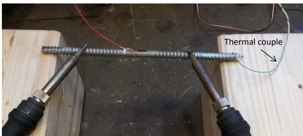
Figure 10 Determination of the thermal expansion coefficient and the temperature effects on the strain gauges
