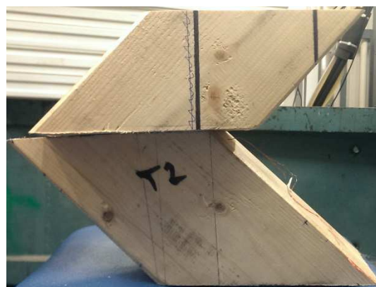
Figure 12 Timber specimens used for double-thread screws
