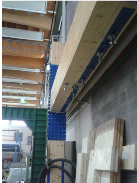
Figure 2 - Glulam reaction frame in the University of Trento's structural laboratory
