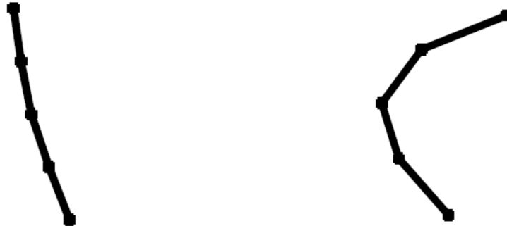
Figure 6 - The first and fourth modes of vibration measured through the height of the building
