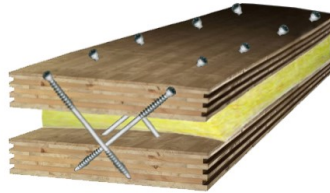
Figure 1: Structural insulated panel composed of cross-laminated timber.
