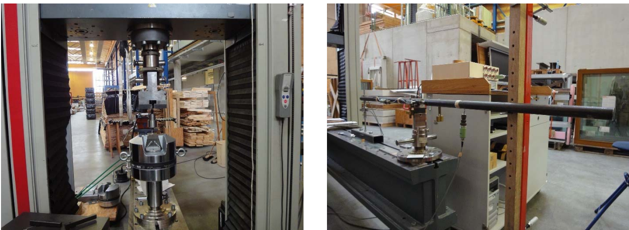
Figure 10: Setup adopted for the uniaxial tension tests (left) and for the bending tests (right).
