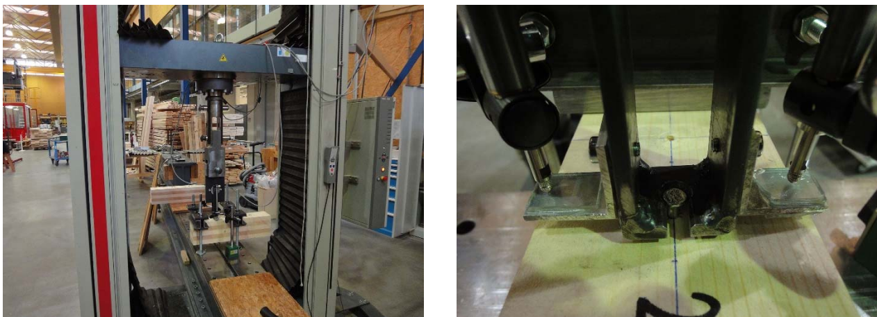
Figure 7: Setup adopted for the withdrawal tests (left) and detail of the fixation (right).
