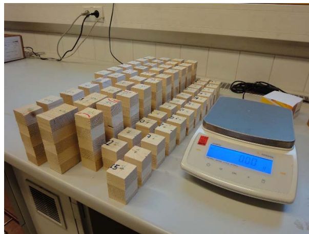
Figure 9: Samples used to measure moisture content and density of the timber.
