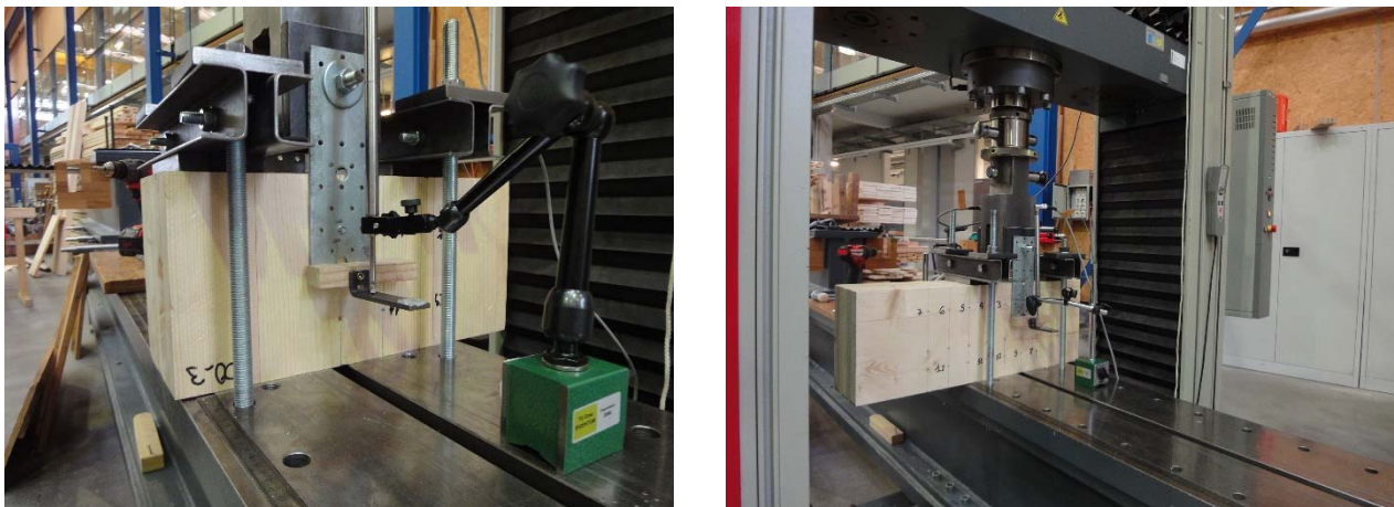
Figure 2: Setup adopted for the shear tests in parallel (left) and perpendicular (right) direction to the face lamination.
