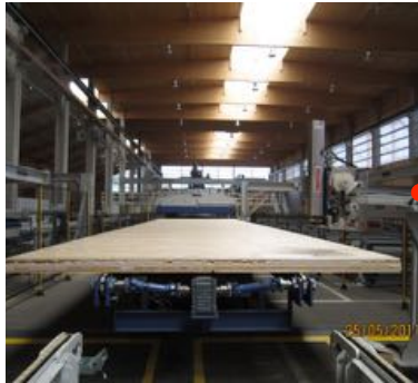
CLT element ready for cutting and joining
