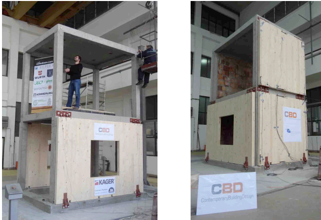
Fig. 3: CLT strengthening system developed in Slovenia
