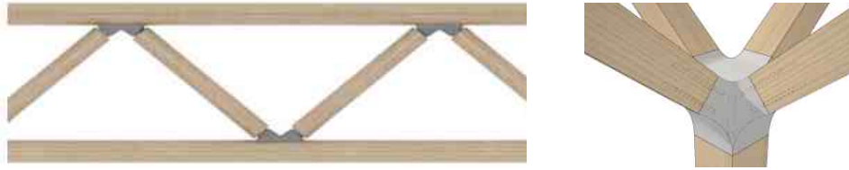
Fig. 1: Examples for unconventional glued applications with concrete-type adhesives: truss structure (left) and tree structure (right)
