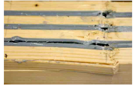
Fig 2b: Fiber buckling of both, timber and CFRP laminates, in the compressive zone.
