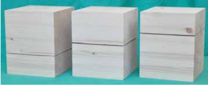
Fig. 5: Glulam test blocks for compressive force measuring in the height of 50 mm, 100 mm and 150 mm.
