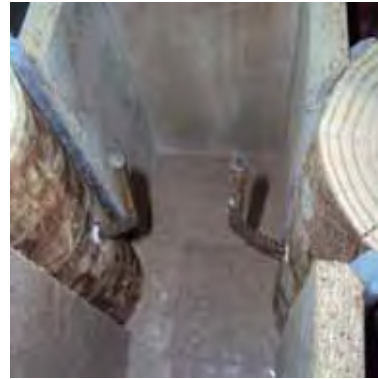
Fig. 3: Dowel connection specimen configuration before cast.
