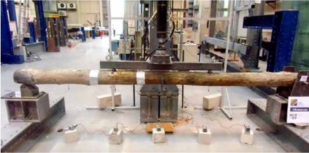
Fig. 1: Setup of bending tests.
