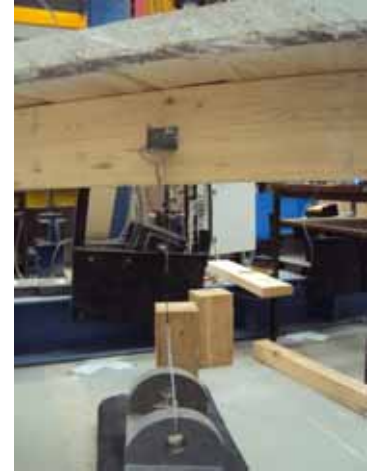
Fig. 4: Dynamic test setup for the beam.
