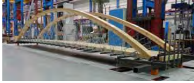
Fig. 5: Bridge with cambered deck
