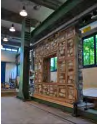
Fig. 1: Cyclic test performed on Casa Baraccata specimen in full scale (left). Cyclic test performed on Gaiola sample (from Poletti et al., 2012).
