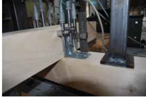
Fig. 4: Spatial joint by steel angle loaded during experiment
