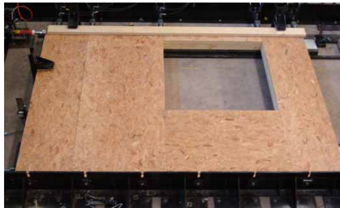
Fig. 1: Racking test apparatus as in EN 594
