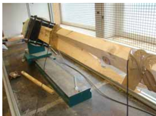
Fig. 3: A typical combined shear tension failure occurred in SP 2.8m joist.
