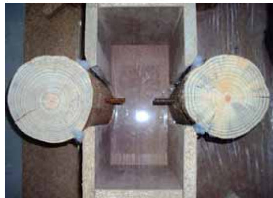
Fig. 1 Dowel connection ready to be cast (top view).
