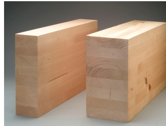
Beech and Spruce glulam with equal strength
