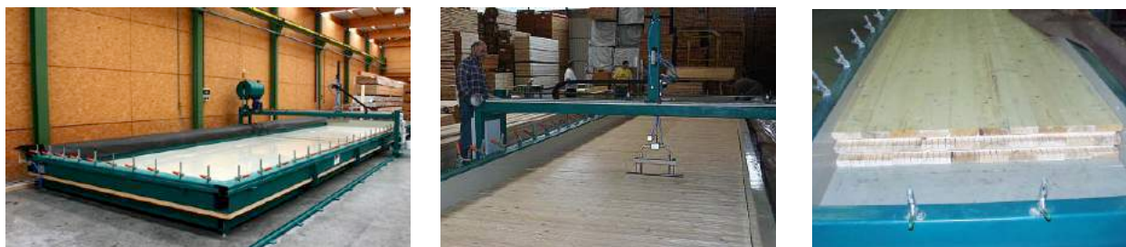
Fig. 8 Vacuum press in combination with an adhesive application system (© woodtec Fankhauser GmbH / CH)
