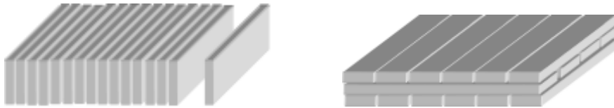
Fig. 4 left fig.: Vertical boards timber panel, nailed or glued; right fig.: CLT, 3 layered
