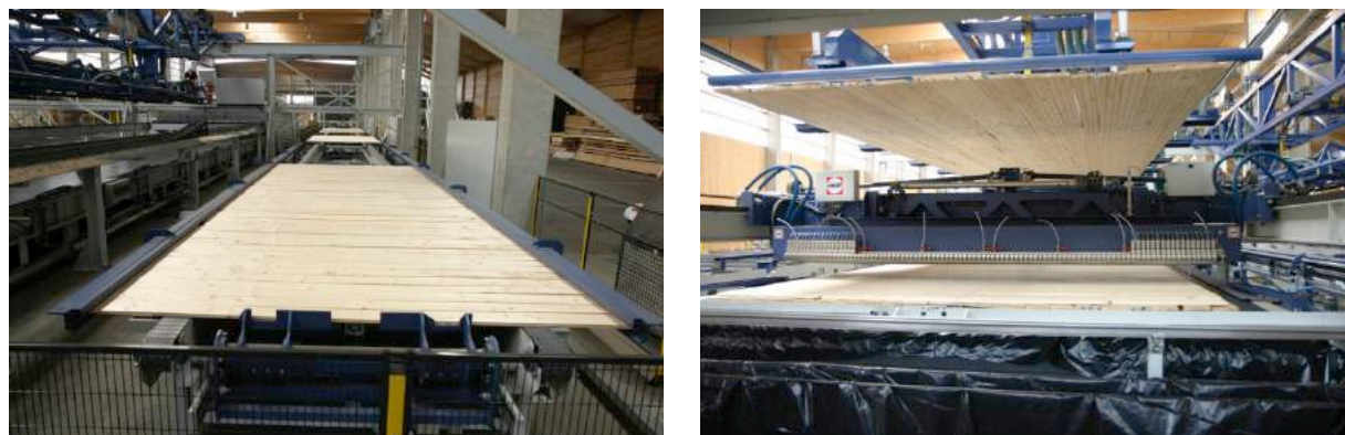
Fig. 6 Placing and aligning of the single layers (left); positioning of layers and application of adhesive (right) (© Minda-Industrieanlagen GmbH / DE)
