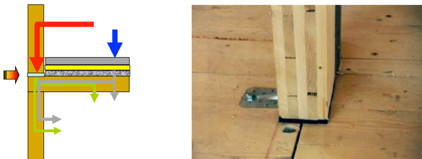
Fig. 78 elastic membrane beyond the wall combined with a floor assembly with high impact sound reduction
