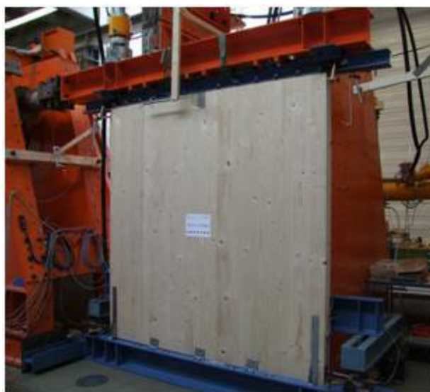
Fig. 1 Test set-up for wall element testing
