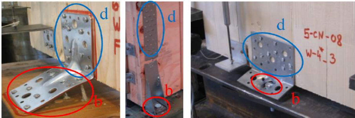
Fig. 23 Undesired failures of CLT connections: yielding of steel part of angle bracket with nails withdrawal (left), failure of steel part of hold-down (middle), pull-through of bolt in the angle bracket (right)
