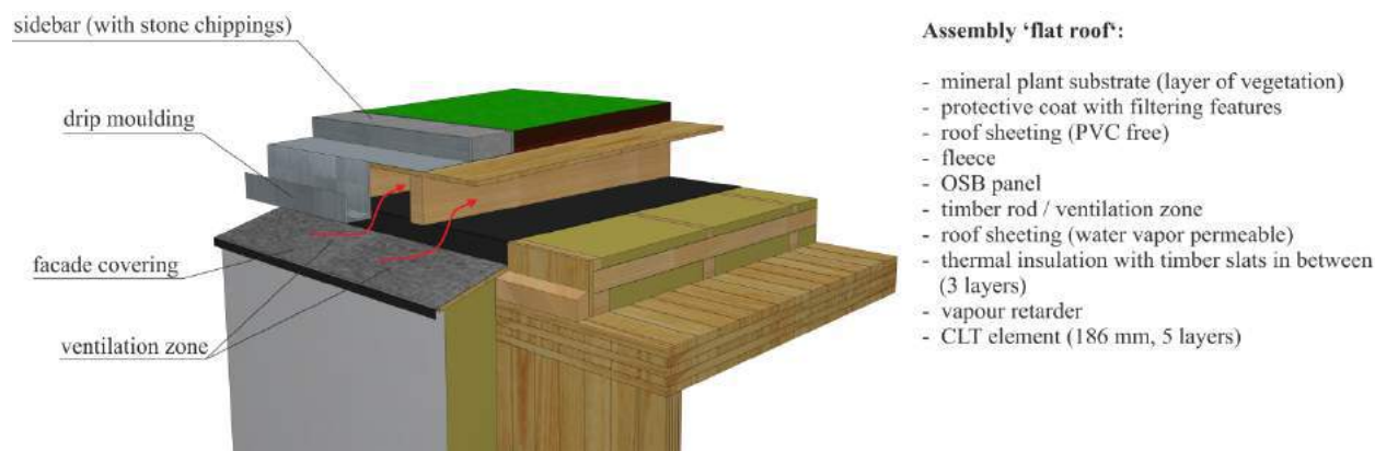
Fig. 12 Assembly of the flat roof construction in CLT
