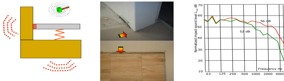
Fig. 73 Effect of an acoustic bridge
