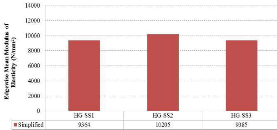
Fig. 12 Edgewise Bending Stiffness
