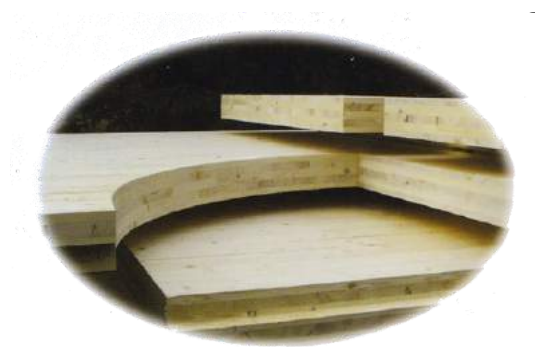
Fig. 1 5-layer panels with different cuts
