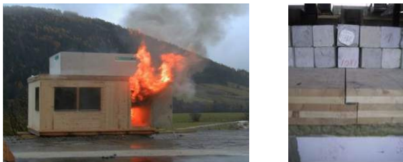
Fig. 6 left fig.: Fire test; right fig.: Standard fire test of a slab with load
