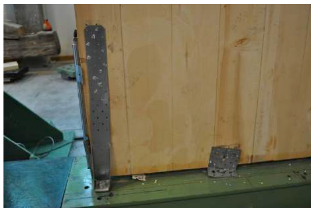
Fig. 2 CLT wall panel at the end of the cyclic tests, near to the failure condition [5]
