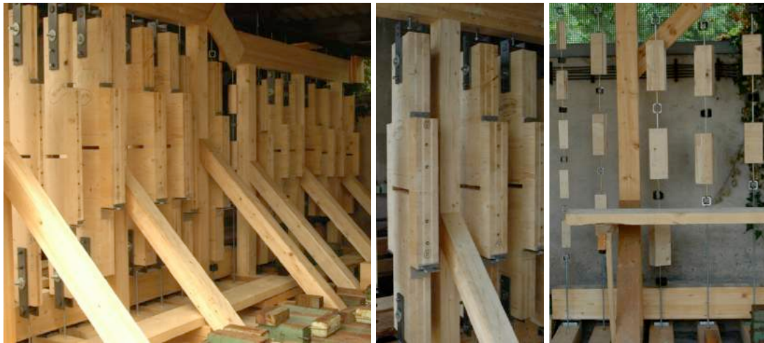
Fig. 16 Long term tests with screwed edge joints in CLT under lateral load and axial load
