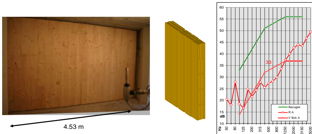
Fig. 63 Left fig.: Sound insulation test facility - Laboratory for Building Physics, University of Technology; Right fig.: Sound reduction index chart of a typical 95 mm 3-layer CLT panel
