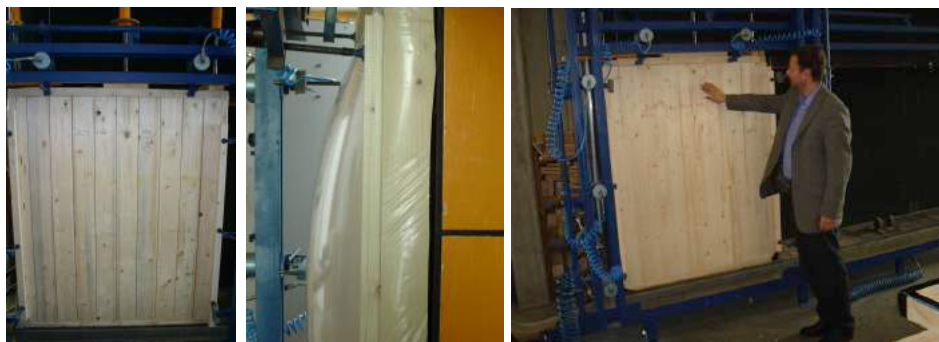
Fig. 48 Test rig for air tightness at the laboratory for Building Physics Graz University of Technology
