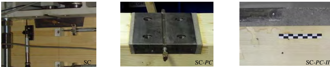
Figure 5: Stud connector placed into the timber with direct contact (SC), filled gap (SC-PC), embedded into PC (SC-PC-II)
