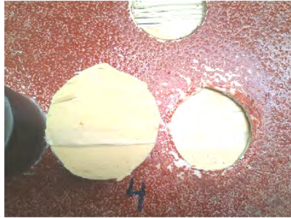
Figure 17: Test specimen with LSS sealant after successful adhesion tensile test [5]
