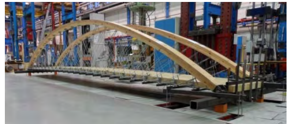
Figure 5: Laboratory model of the bridge
