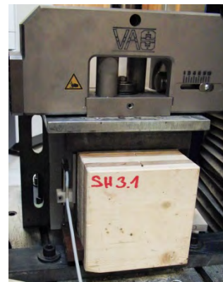
Figure 5: Detail of the test machine readied for a shear test
