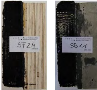
Figure 10: Plastic deformation of a test specimen with PBM sealant on CLT (left) and on concrete (right)
