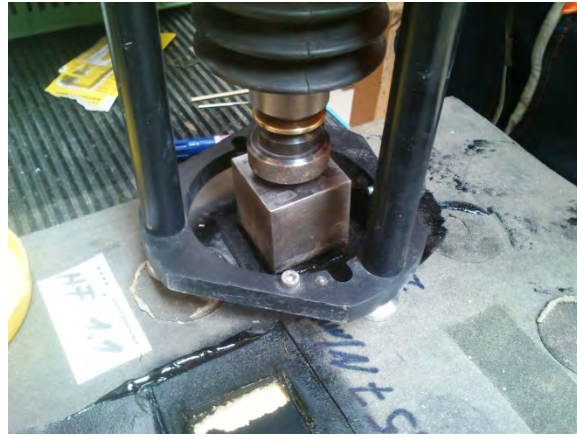
Figure 8: The indenter is pulling at the barely visible PBM sealant underneath it
