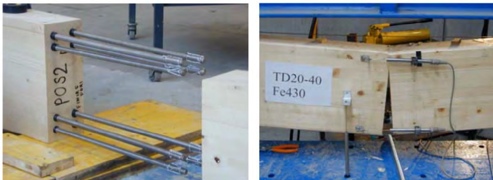
Figure 3: Splice joint with glued-in rods, left: rods glued into one member of the joint, right: plastic deformation of the joint, [9]
