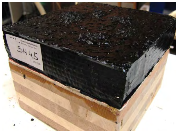
Figure 21: Clear blistering in the surfacing of this specimen of asphalt surfacing on CLT
