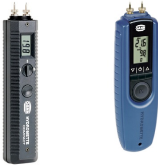
Figure 2: Typical meters with built in electrodes
