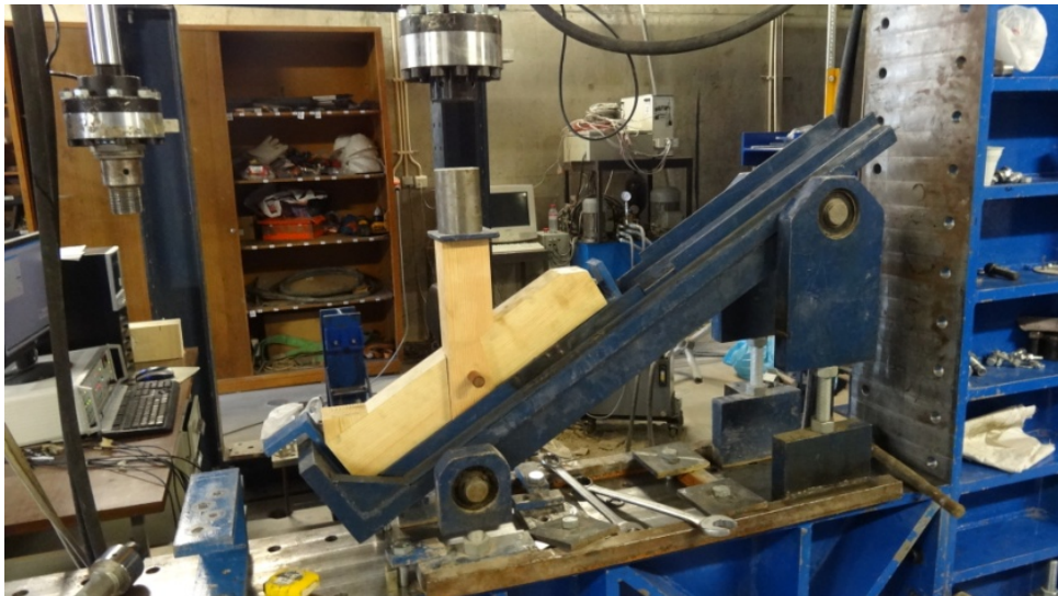
Figure 3: Steel frame used during the experimental campaign of scaled joints
